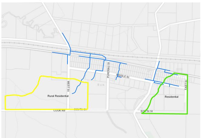
Figure 28: Stormwater network in Pukerau, defined by the blue lines
