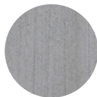
CONCRETE 20MM AGGREGATE BROOM FINISH
