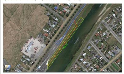
**Figure 2b:** The Section 330 emergency works area on the true right bank. The indicative works area is in green, the indicative access ramp is in red and the progressive direction of works in orange (Map Source: ES Catchment Operations Division).
