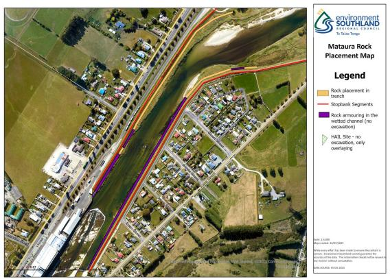
**Figure 2:** The location of the site on an aerial view. The Figure shows the full scope of works along both banks. (Map Source: ES Catchment Operations Division, map created 24 July 2023)<sup>26</sup>.
