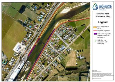
**Figure 2:** The location of the site on an aerial view. The Figure shows the full scope of works along both banks. (Map Source: ES Catchment Operations Division, map created 24 July 2023)<sup>14</sup>.
