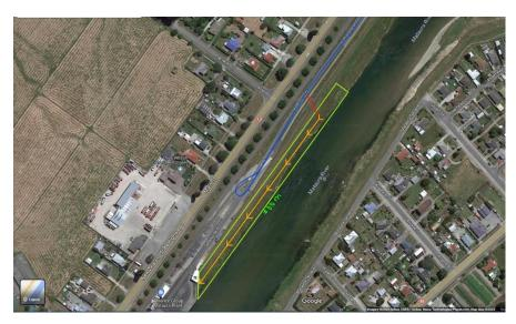
**Figure 2b:** The Section 330 emergency works area on the true right bank. The indicative works area is in green, the indicative access ramp is in red and the progressive direction of works in orange (Map Source: ES Catchment Operations Division).
