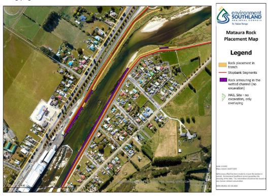
**Figure 1:** The location of the site on an aerial photo and the proposed works along both banks. (source: Extract from Figure Appendix E-1, submitted with the application).
