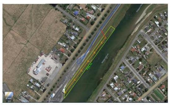
Figure Appendix E-1b: The Section 330 emergency works area on the true right bank. The indicative works area is in green, the indicative access ramp is in red and the progressive direction of works in orange (Map Source: ES Catchment Operations Division).
