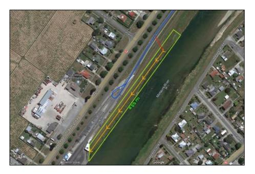
**Figure 2:** The Section 330 emergency works area on the true right bank. The works area is in shown in a green outline, the access ramp is in red and the progressive direction of works is in orange. (source: Extract from Figure Appendix E-1b, submitted with the application).
