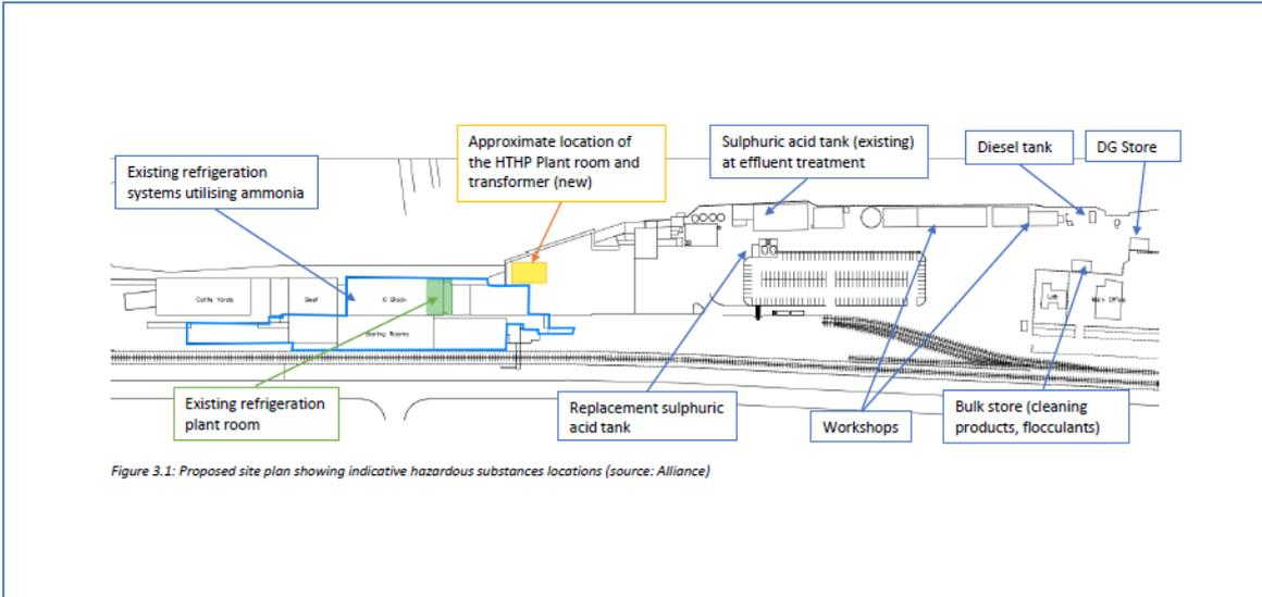
**Figure 1. Proposed site plan showing approximate location of proposed HTHP Plant room and hazardous substances locations**
