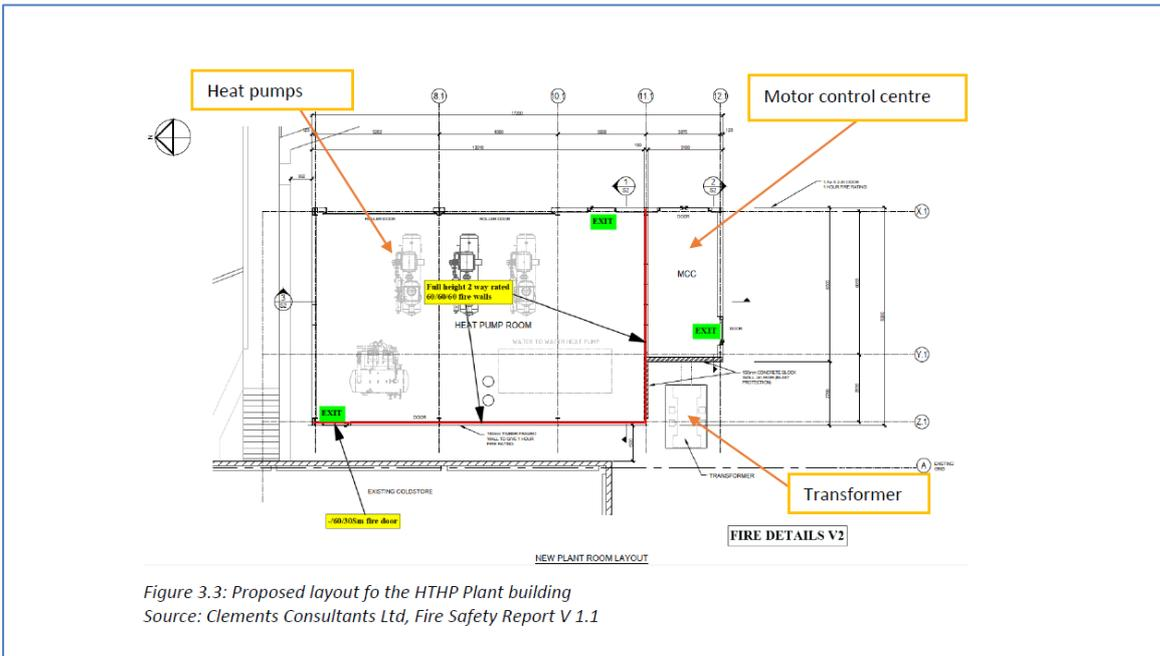
**Figure 2. Proposed floor plan of HTHP Plant room including HTHP's and Transformer**
