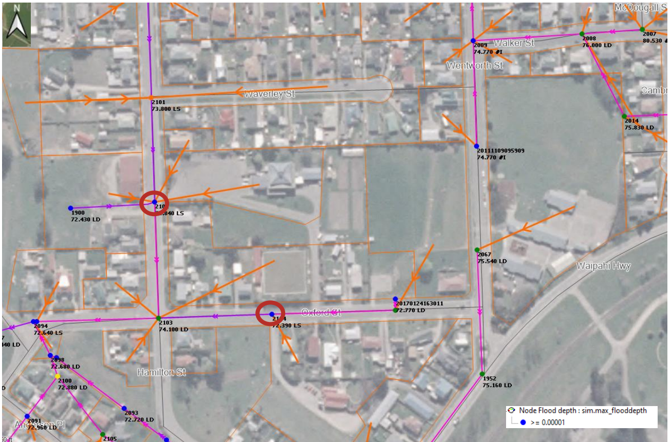
Figure 6-3 Surcharged wastewater pipes and overflow points around the new development.
