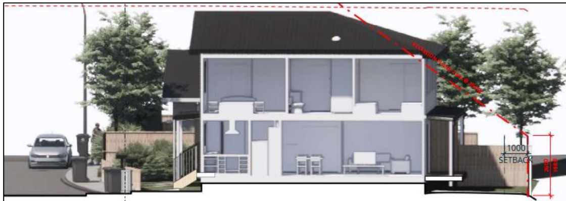
Figure 6 – Image Depicting Extent of Recession Plane Breach for Units 22 and 23 (Source: Appendix 3 ).
