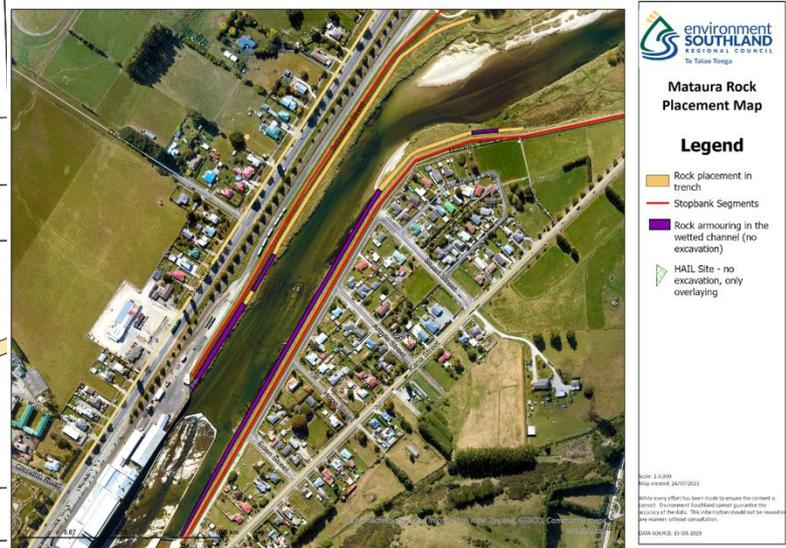
Figure 2: The location of the site on an aerial view. The Figure shows the full scope of works along both banks. (Map Source: ES Catchment Operations Division, map created 24 July 2023).
