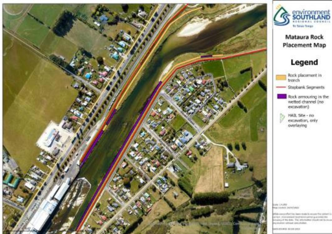
**Figure Appendix E-1:** The location of the site on an aerial view. The Figure shows the full scope of works along both banks. (Map Source: ES Catchment Operations Division, map created 24 July 2023)<sup>63</sup>.
