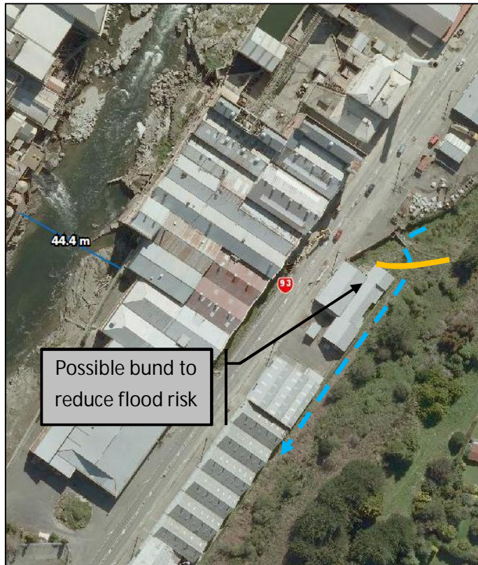
Figure 5: Potential secondary flowpath from the Waikana Stream that could endanger the building floor level of 116-130 Kana Street
